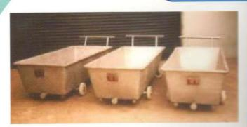
Butter prepared in the churn requires unloading. Hence, a hygienically designed stainless steel open type trolley is required. The size of trolley should be such that it should accommodate all butter from the churn. If the quantity of butter made is less, one may collect butter in other containers, provided they are clean and designed to handle food products.
