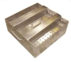
Used for holding the curd in preparation for pressing the curd and shaping the finished paneer, Stainless steel is used for fabrication of moulds.
