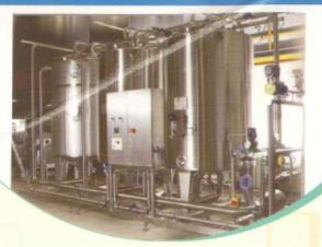
It is a process that combines high velocity scrubbing and chemical actions of the circulating detergent solutions to remove the deposits from milk handling equipment. The clean-in-place (CIP) system of cleaning eliminates the dismantling and reassembling process for the equipment for the cleaning purposes. This reduces the human effort involved and economizes on labour, time and energy.
