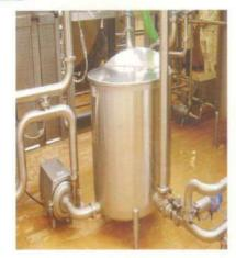
Application: Balance tank is required to receive &
